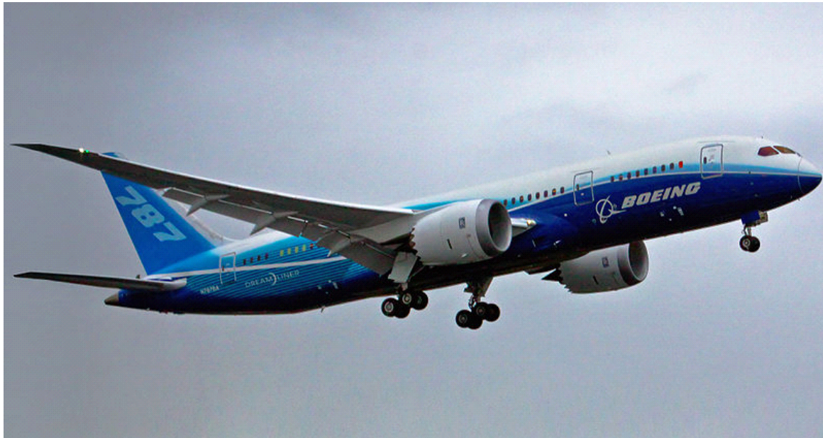
Figure 2: A Boeing 787 is constructed of up to 50% composite materials 2
